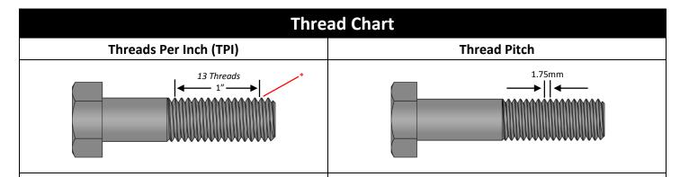
When ordering or referencing inch fasteners, **Threads Per Inch** (TPI) is used instead of the thread pitch.
